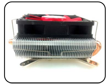
1.5U low height design cooler for slim type cases.
